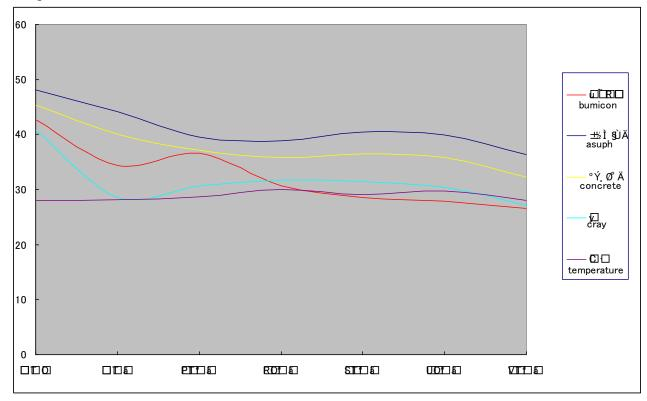
Surface temperature of BUMICON can be cooler than concrete by as much as 8 °C, and asphalt by as much as 12 °C
